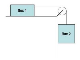
ANSWER: The free body diagram for Box 1 has  $m_1g$  (down),  $F_N$  (up),  $F_T$  to the right and  $F_{friction}$  to the left. For Box 2 we have  $m_2g$  (down) and  $F_T$  (up). The  $F_T$ 's are the same (in magnitude).
